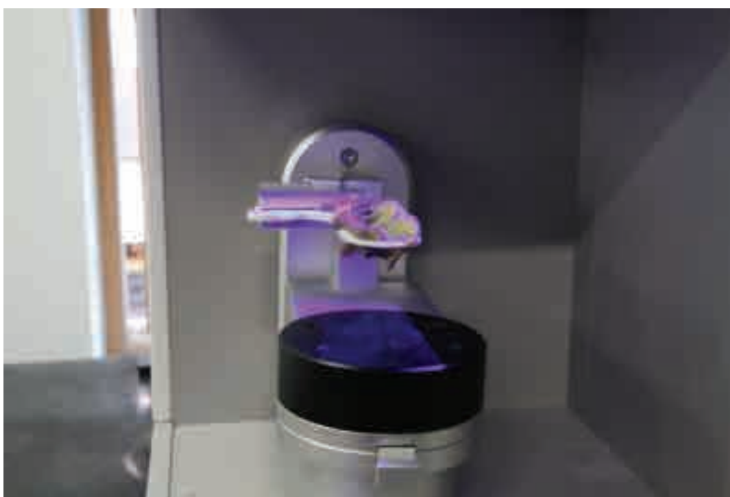
Put the impression jig and mount onto the scanner. Click "Auto Scan" 2 to proceed with scanning
